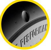
The introduction of a dimple indicator moulded into the sidewall in three places gives an early warning the driver that the sidewall rubber may have been "scrubbed" enough to consider a tyre change if the barrier is compromised by excessive wear or damage.
